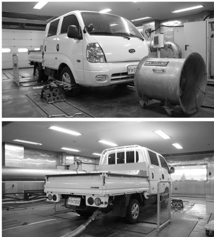
Fig. 12 Performance test of DME truck (NEDC mode)
