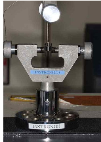
Fig. 2. Pull out test in universal test machine.
