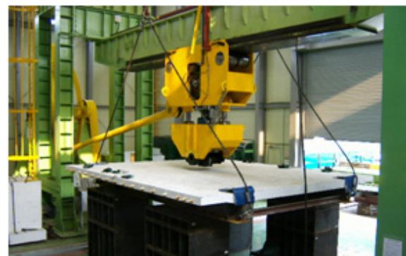
Fig. 2 Static loading test
