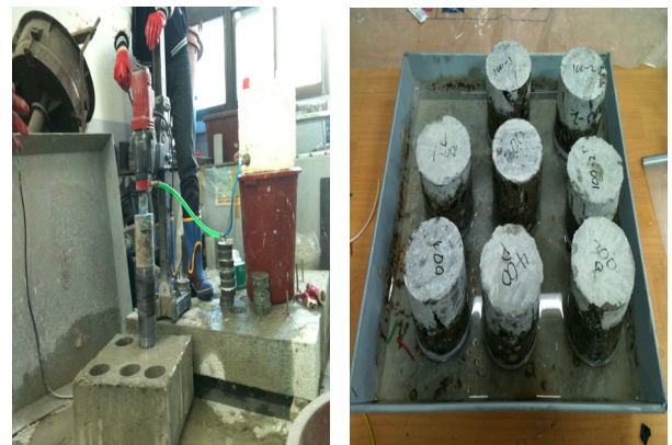
Fig. 6 View of coring and amount of water absorption
