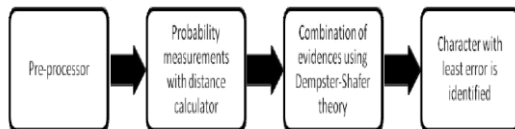
Fig. 4. Block Diagram of offline handwritten Urdu character recognition system.
