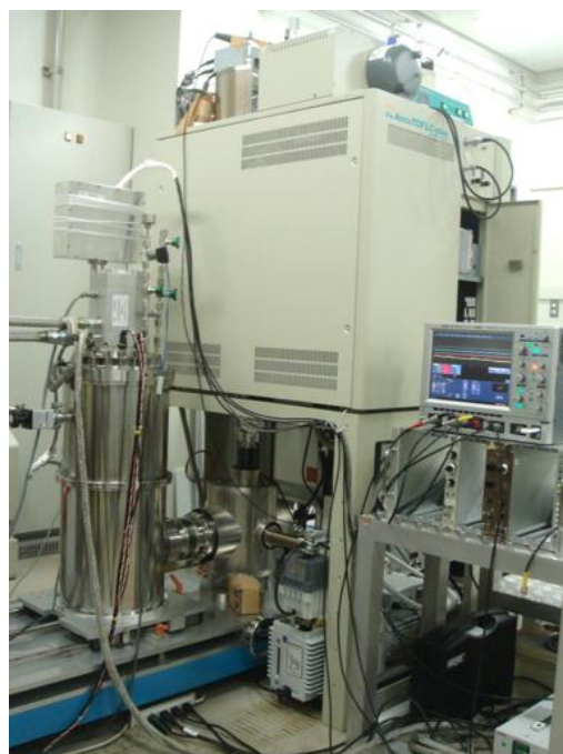
Fig. 3. ESI TOF MS equipped with STJ array detector with 100 pixels. The detector is cooled by the cryogen-free 0.3 K cryostat on the left hand side.
