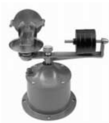
Fig. 1. Centrifugal casting machine
