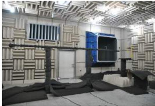
Fig. 3. Microphone Line Array for Noise Test
