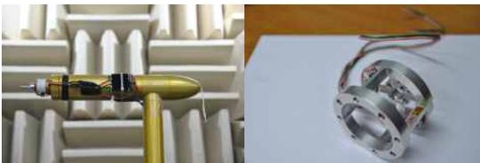
Fig. 2. Rotor Test Jig & 2-Axis Balance
