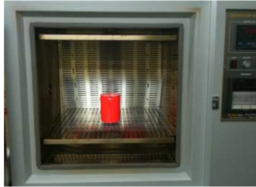
Fig. 13. Low temperature fire test apparatus
