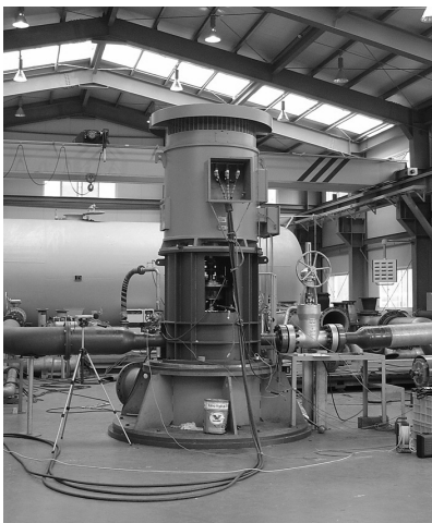
Fig. 14 Pump test setup
