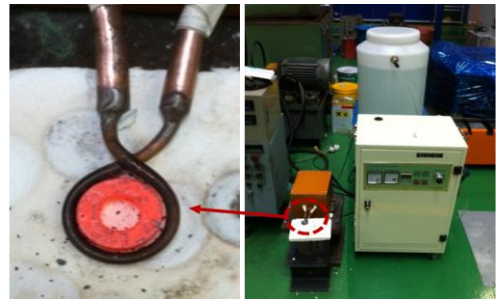
Fig. 7 The experiment using high frequency induction heating furnace
