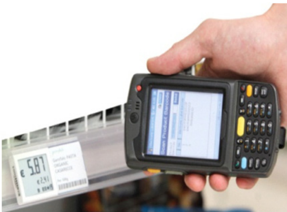
Fig. 6 Example: Reading an NFC tag embedded in an electronic price marker with a smartphone
