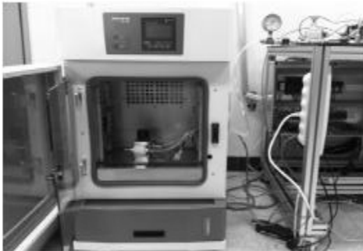
Fig. 5. Blower operation in chamber for worst stress condition test.
