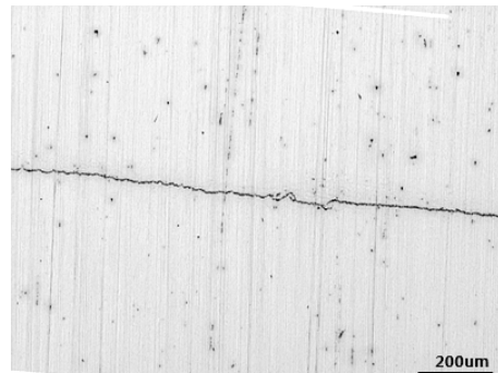
Fig. 4 Centerline cracking of 25mm thickness specimen(3% plastic stain) after HIC test
