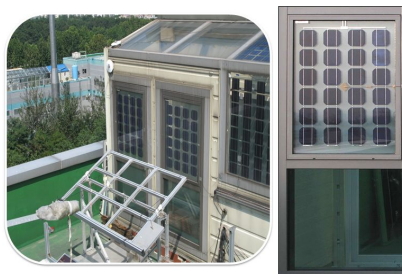
Fig. 5 BIPV experimental model of G/G (2) type
