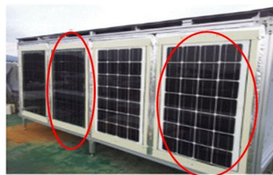
Fig. 4 BIPV experimental models(left circle: G/G(1), right circle : back sheet type)
