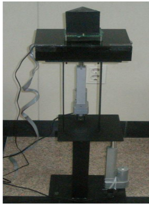
Fig. 6 The solar tracker with two degree of freedom
