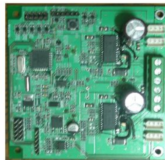
Fig. 5 Solar tracking control board
