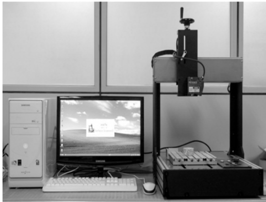
Fig. 4. The laser profiler which was used for roughness measurements
