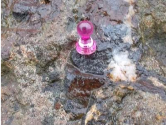
Fig. 6. Close view of the magnetite ore at P1, Mulgeum deposit. Magnet in pink is 1 cm in length.
