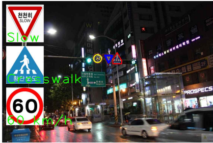
Fig. 6. Experimental results of recognition for various shapes of traffic signs in a rainy night.
