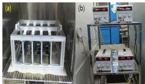
Fig. 5. (a) Fixed Jig for Life Test Board and (b) Power Supply
