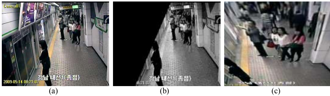
Fig. 4. (a) Original image (b) Result of image after setting ROI (c) Spatially transformed image
