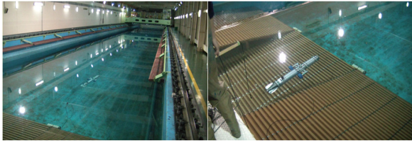
Fig. 4. Towing tank and the underwater robot for the experiment
