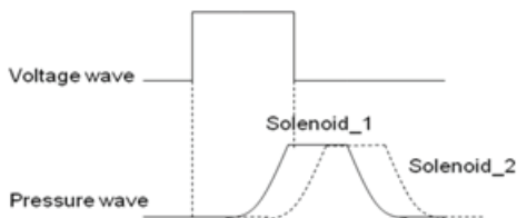
Fig. 2 Operating characteristics of solenoid operated pneumatic valve
