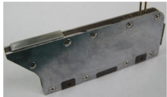
b) Manufactured air ejector with a piezoelectric actuator Fig. 4 Piezoelectric actuator and an air ejector
