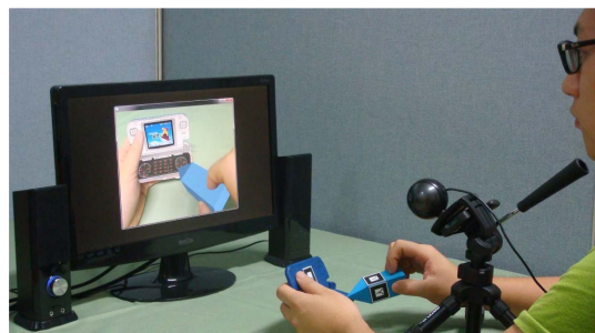
Fig. 1 Design evaluation of a handheld product using AR-based tangible interaction
