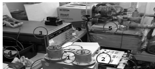
Fig. 2. Capacitance measuring devices: ① -Filter-sensor, ② -Sensor controller & monitoring system, ③ -Impedance analyzer, ④ -Data logger and ⑤ -Engine lubrication system rig tester.
