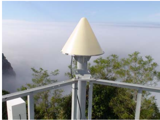
(b) ChokeRing Antenna at Ulleungdo Station
