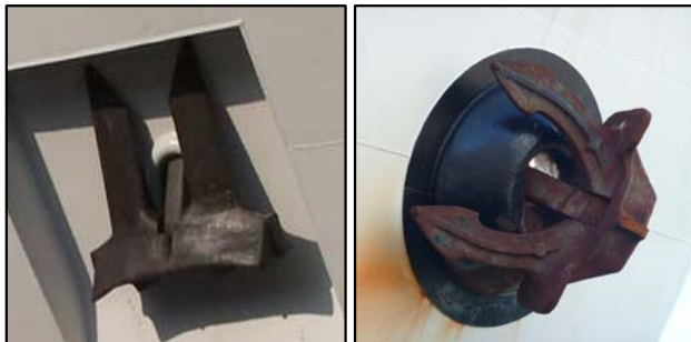
Fig. 1 AC-14 type(left) & ASS type(right) anchor
