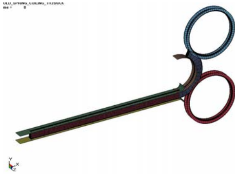
Fig. 6 Finite element model for coiling analysis
