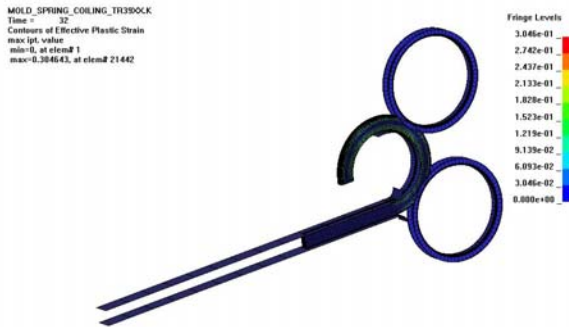
Fig. 7 Effective plastic strain distribution of the R39 coiling result
