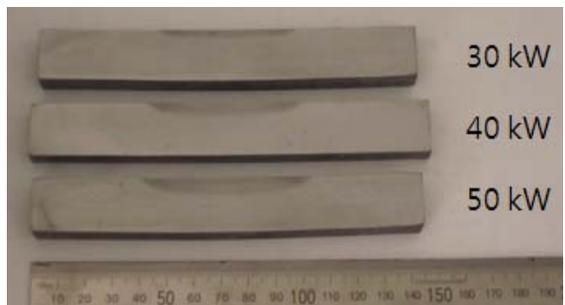
**Fig.14** Numerically calculated temperature distribution along the thickness direction exhibited together with heat affected zone obtained from actual high frequency induction heated samples under different input power conditions
