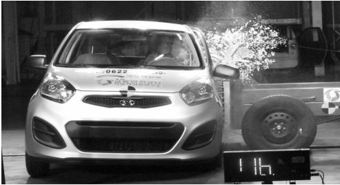
Fig. 3 Impact moment of Kia Morning at side impact test
