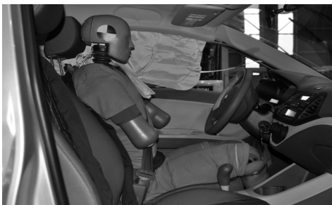
Fig. 5 Deformed shape of side structure and interior of Morning after side impact test
