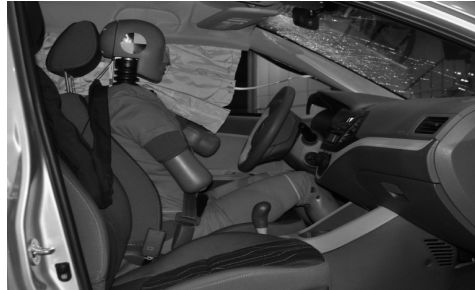
Fig. 6 Deformed shape of side structure and interior of Morning after pole side impact test
