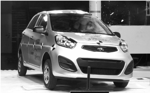
Fig. 4 Impact moment of Kia Morning at pole side impact test
