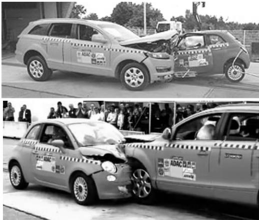
Fig. 1 Frontal car-to-Car crash (FIAT 500 vs. AUDI Q7); 56kph, 50% overlap ratio of small car
