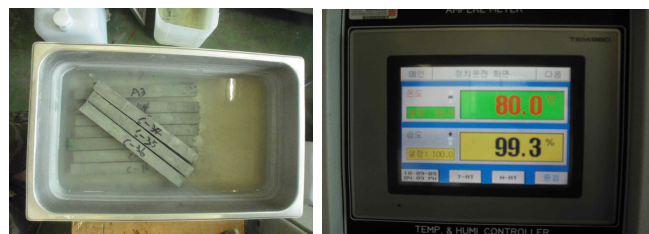
Figure 6. Specimens and equipment for immersion expansion in 80 °C water
