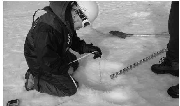
Fig. 2 Measurement of ice thickness
