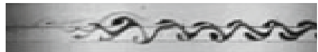
Fig. 1 2D Karman vortex in lee of towed obstacle in stably stratified fluid (Voropayev & Fernando, 1996)
