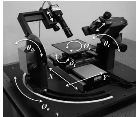
Fig. 1. Laser scattering inspection mechanism.
