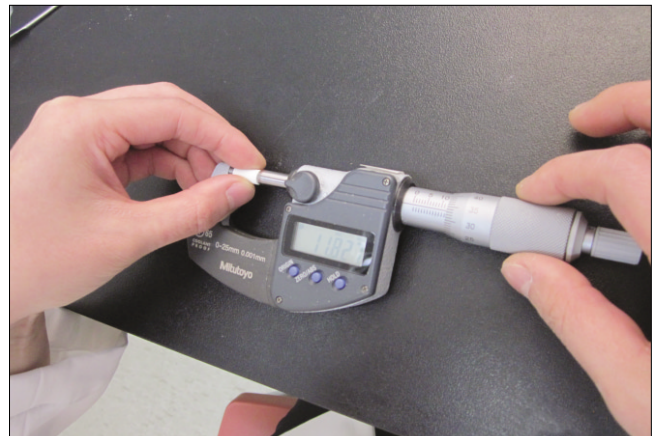
Fig. 3. The length measurement using the micrometer.
