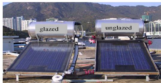
그림 5. PV/T collectors with and without glass cover<sup>34)</sup>
