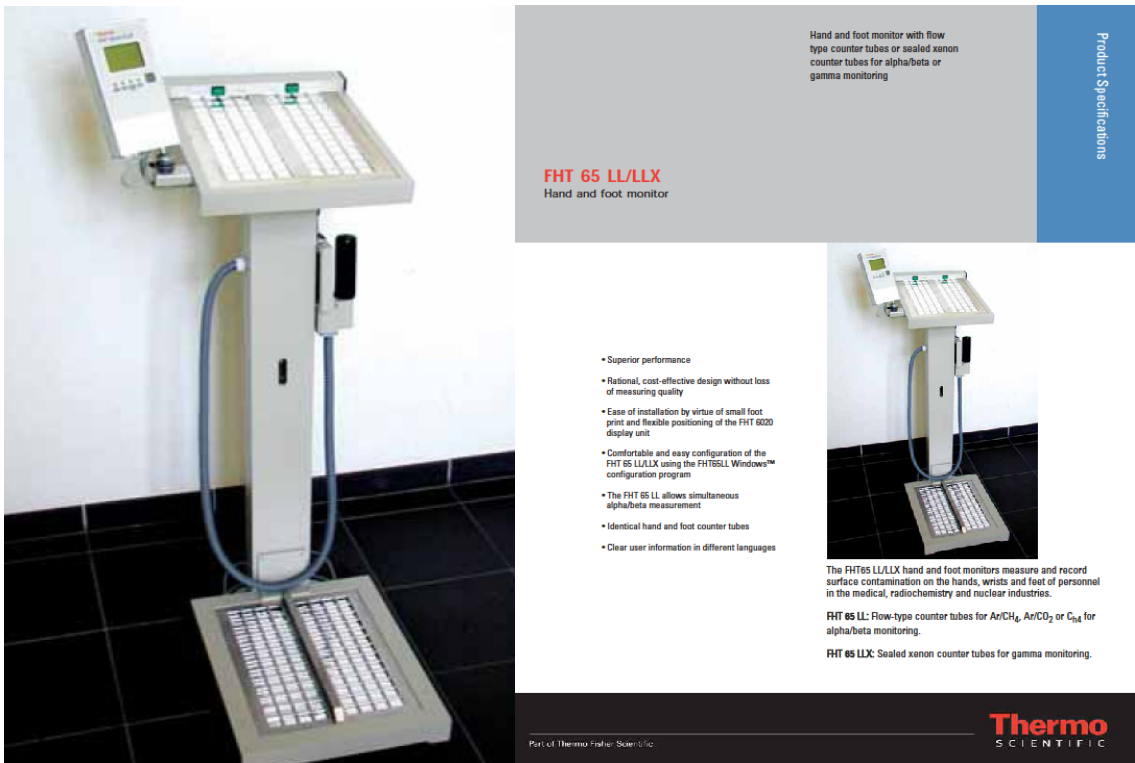
Fig. 1. FHT 65 LLX ; Size (in operation): Approx. 1400 H x 380 W x 750 D mm (55" H x 15" W x 29.5" D), Weight: 35 kg (77.2 lbs), Ambient temperature: +5 °C to +50 °C (41 °F to 122 °F), Relative air humidity: 10 % to 90 % (non-condensing), Protection system: IP30, Voltage: 85 to 285 VAC (47 to 63 Hz), Power requirements: < 10 W, Display ranges: 0.01 to 1000 s -1 (0.01 to 1000 Bq/cm 2 ).
