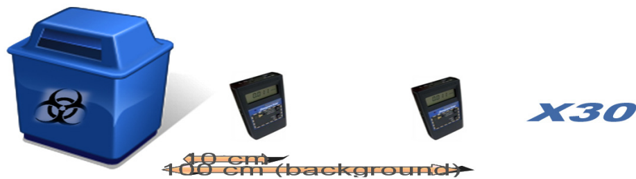
Fig. 2. This picture shows the measurement by using survey meter detectors.
