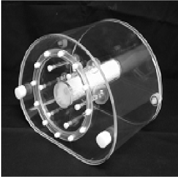
Fig. 1. This is NEMA IEC PET body phantom which consists of a body phantom, a lung insert and 6 fillable spheres (diameter: 10, 13, 17, 22, 28 and 37 mm).
