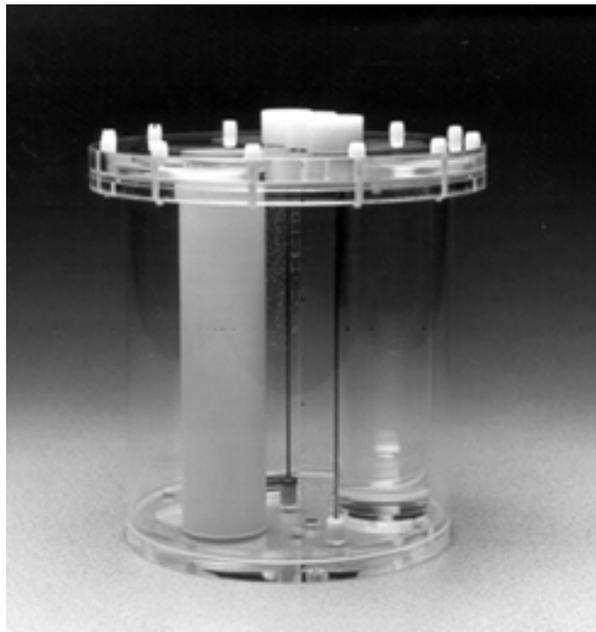
Fig. 2. This is NEMA PET phantom which consists of 3 fillable spheres (diameter: 50 mm).
