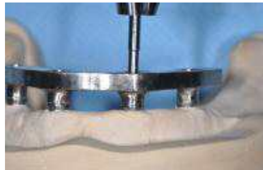
Fig. 6. Measurement of detorque values (HTG2-200Nc, Imada Co., Toyohashi, Japan)
