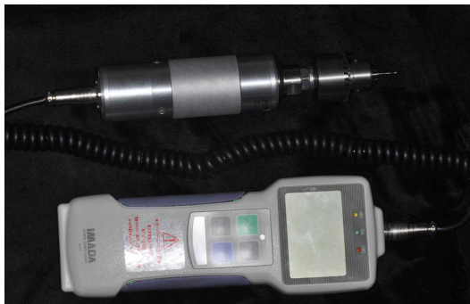
Fig. 5. Digital torque gauge (iSD900, Nakanishi Inc., Tochigi-ken, Japan)
