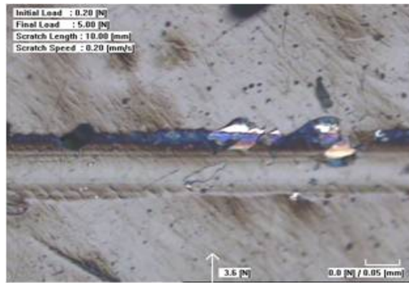
Figure 2. Optical microscope image of scratch test in DLC coated Ni plate.
