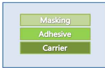
Figure 1. The base structure of single coated tape.
