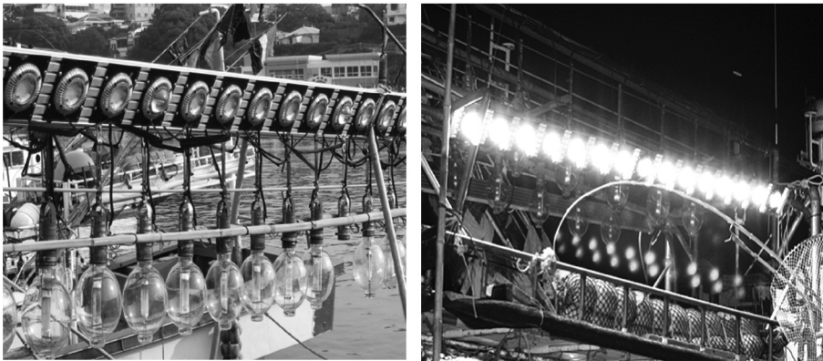
Fig. 2. Squid jigging boat established LED light system (Jaeun-ho).
