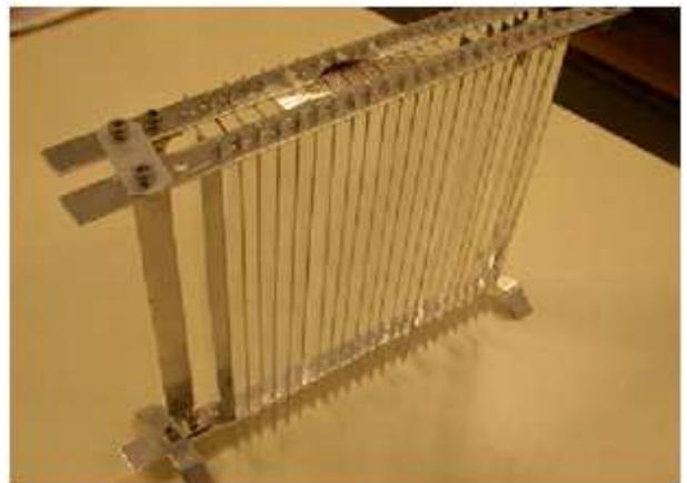
Fig. 4 Azimuth collector blinds
