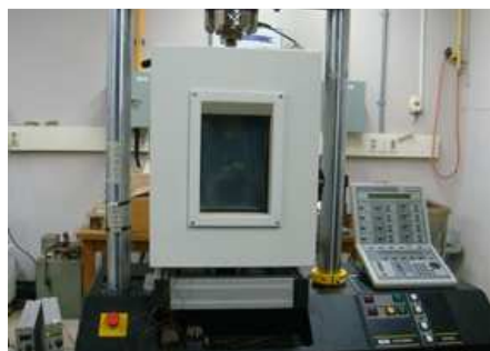
Fig. 3 Fretting fatigue test apparatus at 320°C
