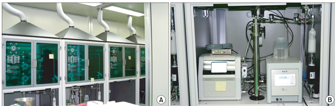
Fig. 2. Nose-only inhalation chamber (A), Scanning Nano-particle Spectrometer and Condensation Particle Counter (B).
