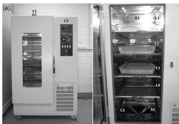
Fig. 1 An automatic brown rice germinating system of air-phase type with anion radiation and intermittent water spraying: image of front view (A); image of inside view (B).
