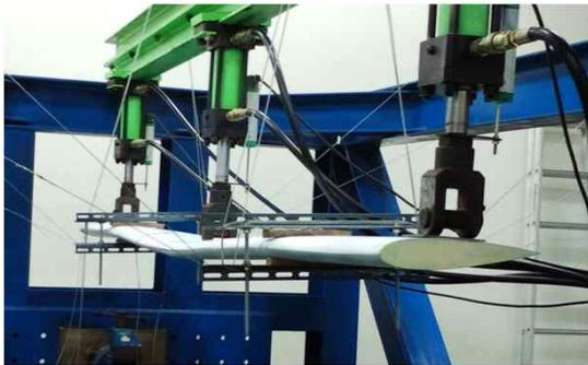
Fig. 9. Static test of the prototype blade
